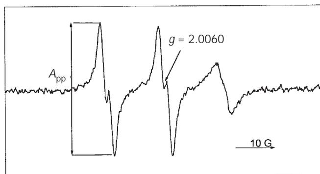
FIG. 1. Electron spin resonance spectrum of the spin-trap *N*-*t*-butyl- $\alpha$ -phenylnitron in rapeseed oil after 278 min at 70°C. The *g*-value was determined to be 2.0060. The peak-to-peak amplitude  $A_{pp}$  is determined as shown.
